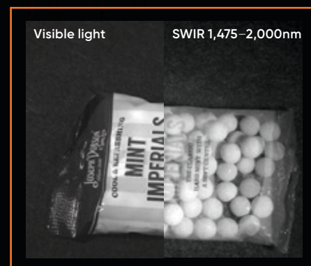
Two images of a packet of sweets – on the left is the image under visible light, and on the right is the image using a SWIR enabled camera with the sweets clearly visible.
